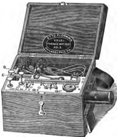
FIG. 50. —The VOLA FARADIC BATTERY.—A, platform; B, switch for putting battery in action and out of action; C, contact screw-lever functioning rapid and slow interrupter; D, rapid vibrating interrupter; E, slow interrupter; F, switch for selecting the primary or secondary induced currents; G, commutator; H, governing handle for graduating both secondary and primary currents; I, guide and index indicating position of coils; K, movable secondary induction coil.
