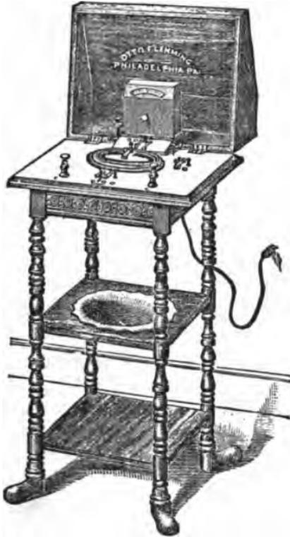
**FIG. 8.—BEDSIDE GALVANIC TABLE.**—For use with supply wires from an incandescent plant or permanent battery. Connection with the supply wires is made by a double plug and socket, or by two binding posts.
