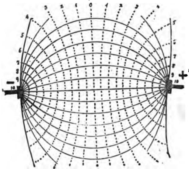
**FIG. 47.—DISTRIBUTION OF A CURRENT OF TWENTY VOLTS WITHIN THE HUMAN BODY.**—The equipotential lines or planes become segments of perfect circles, and the lines of flow, necessarily crossing the latter at right angles, become greatly curved and extend to all parts of the body in passing from pole to pole. The number of milliamperes traversing the lines of flow differs somewhat, being inversely proportional to the length of the lines.
