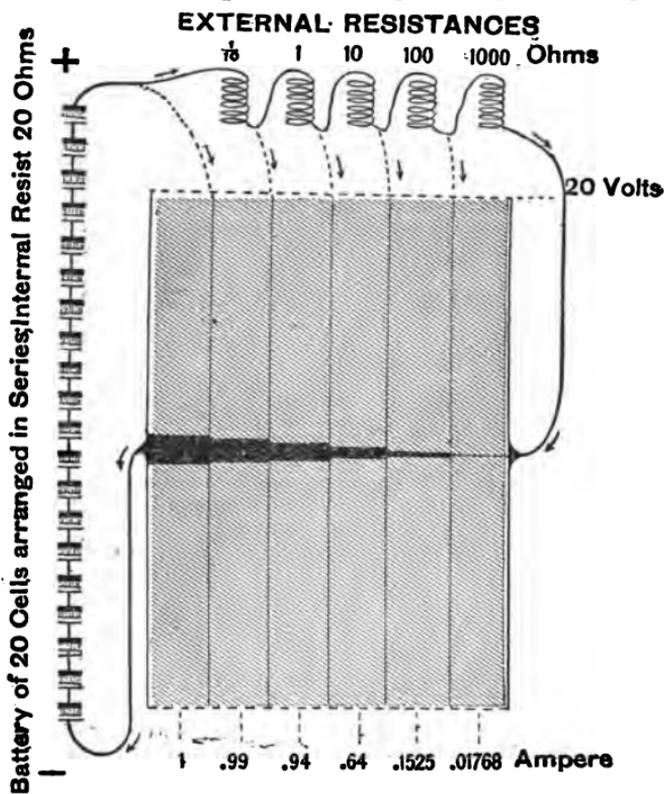
FIG. 44.—GRAPHIC DELINEATION OF THE VOLUMES AND PRESSURE OF CURRENTS FROM A BATTERY OF TWENTY CELLS ARRANGED IN "SERIES."—The battery has an electromotive pressure of twenty volts and an internal resistance of twenty ohms. The heavy shading in the first five imaginary current sections shows the exact proportion of volume on the scale of the preceding cuts. The space allotted to represent pressure is reduced to one-half the scale adopted in Figs. 42 and 43 for purposes of convenience.
