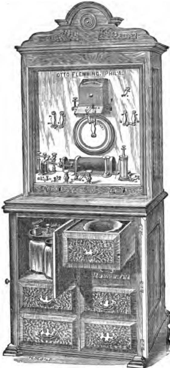
FIG. 10.—THE AUTHOR'S OFFICE CABINET.—This cabinet furnishes both currents, separate or combined. Permanent cells may be placed on shelves attached to the rear of the cabinet, and the whole mounted on rollers; but usually the larger size of cells are to be preferred, kept in a separate compartment. The original form of the graphite or pencil-mark controller is shown in the centre of the switch-board.
